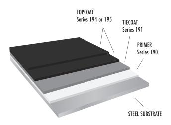
SERIES 194 HULLCLAD CU A tin-free, antifouling paint with self-polishing action for service against marine growth and organisms. This coating's specific chemical composition provides an advanced fusion technology during operation, resulting in reliable antifouling performance and options for extended drydock intervals. Designed for optimum performance for up to 36 months.
