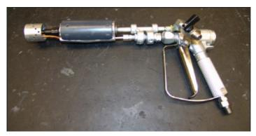
**Note:** Pump assembly should include a moisture trap and oiler, air regulator with gauge and fluid outlet drain valve and outfitted with a gravity fed material hopper (material will not feed through a suction tube).
